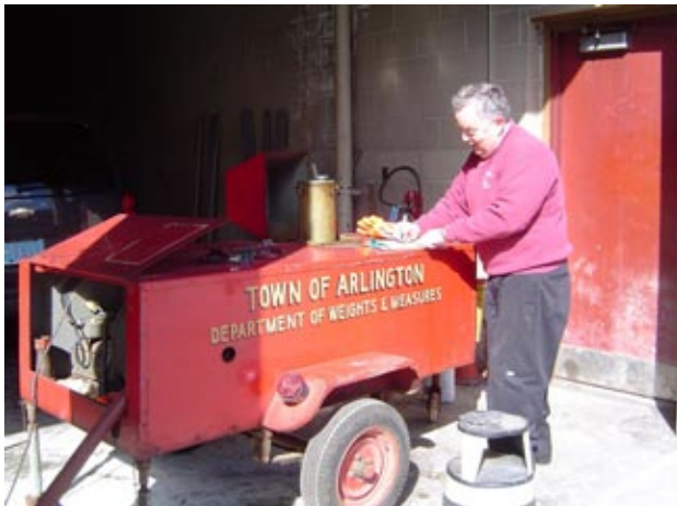
Sealer of Weights and Measures with the oil truck gallon measuring device
