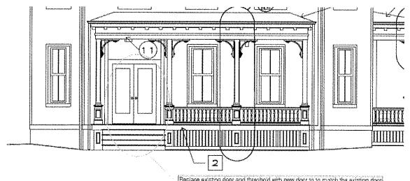
Replace existing door and threshold with new door to to match the existing door match the existing door and challes. Existing Hardware to be reused.
