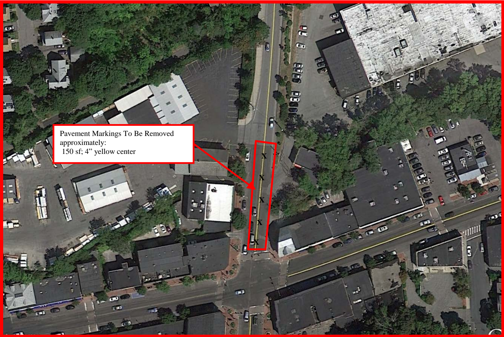
Pavement Marking Removal Area: Sketch #2
