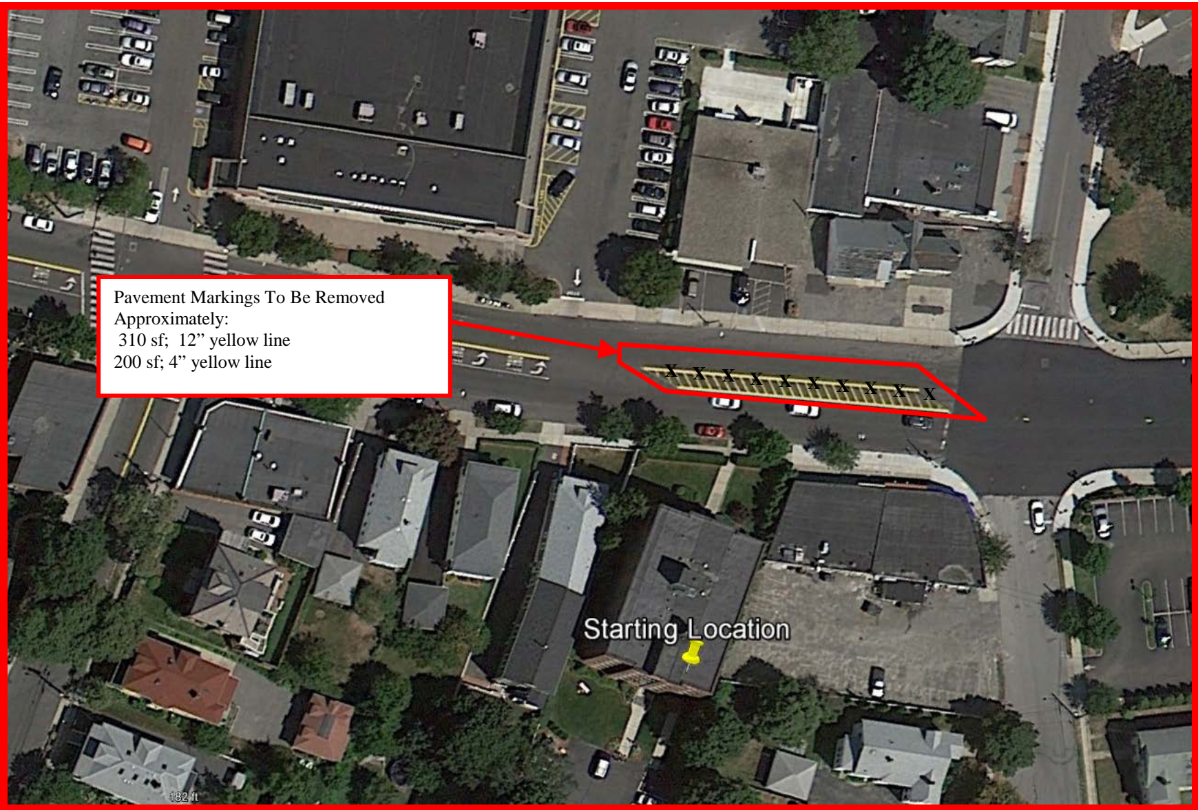
Pavement Marking Removal Area: Sketch #1
