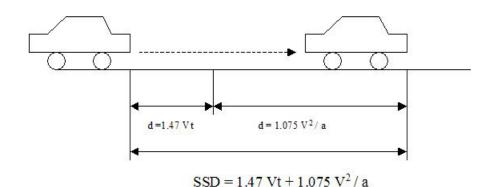
Combining the brake reaction distance and the braking distance as illustrated in the illustration to the right provides the following formula:
