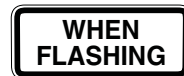
Substitute Lower Plaque (MUTCD S4-4) (for use where flashing signs are installed)
