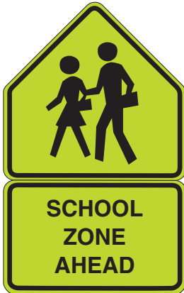
School Speed Limit Advance Warning (MUTCD S4-5)
