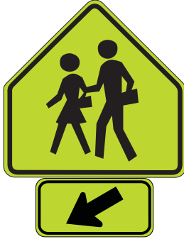
School Crosswalk Warning Assembly (MUTCD S1-1) (MUTCD W16-7p)
