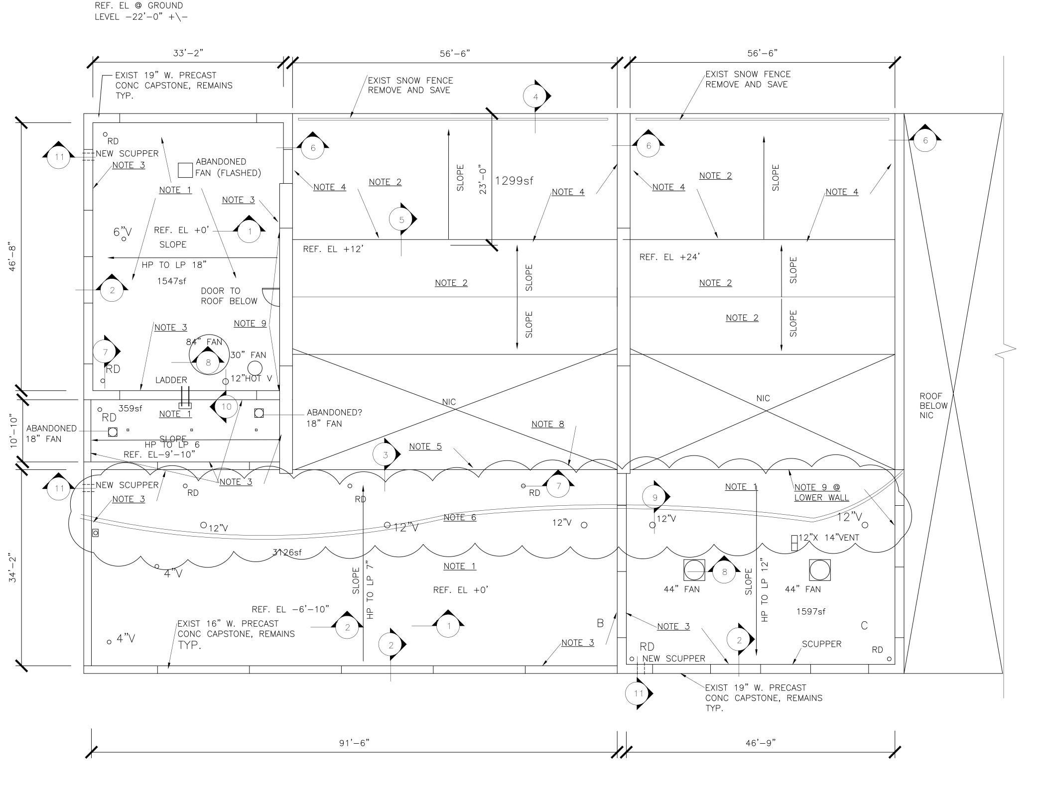
NOTE 1 EXISTING BUILT UP FLAT ROOF, REMOVE ENTIRELY INCLUDING MEMBRANES, INSULATIONS, VAPOR BARRIERS, STONE BALLAST AND ANCHORS. CLEAN AND/OR SCARIFY EXISTING STRUCTURAL CONCRETE OR GYPSUM DECKS. CLEAN
