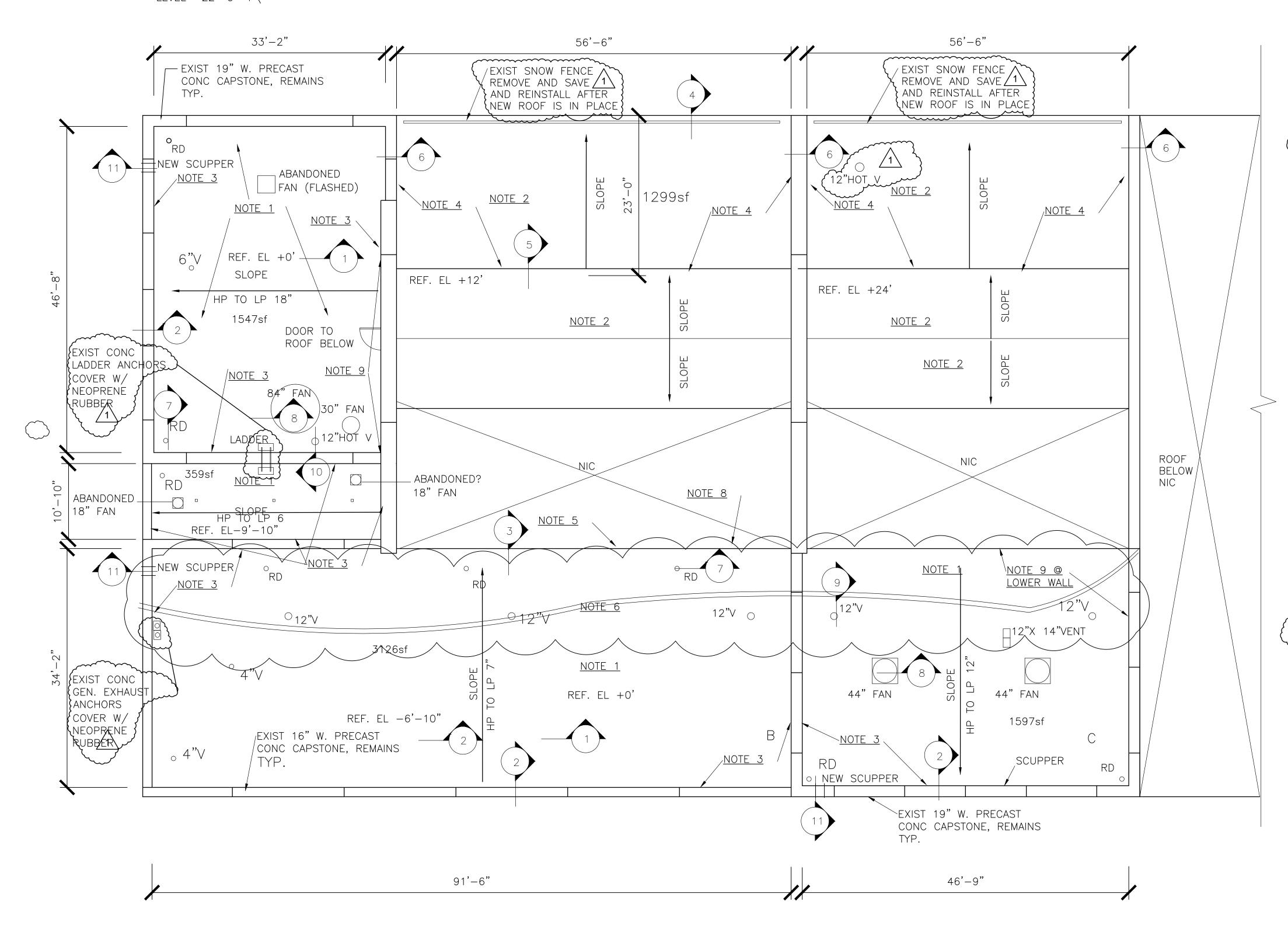
NOTE 1 EXISTING BUILT UP FLAT ROOF, REMOVE ENTIRELY INCLUDING MEMBRANES, INSULATIONS, VAPOR BARRIERS, STONE BALLAST AND ANCHORS. CLEAN AND/OR SCARIFY EXISTING STRUCTURAL CONCRETE OR GYPSUM DECKS. CLEAN METAL DECKS. INSTALL NEW BUILT UP ROOF AS SPECIFIED.
