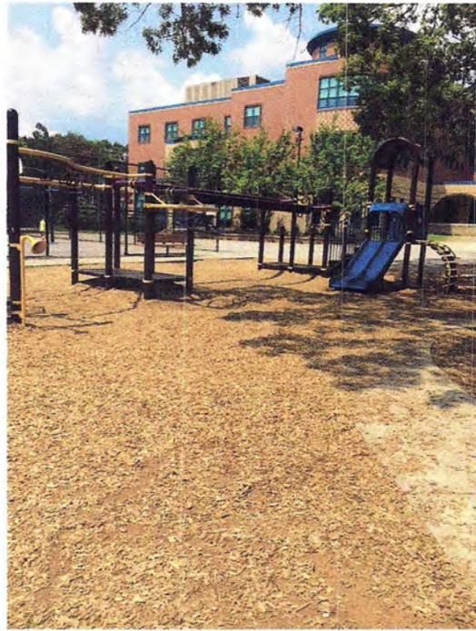
A surfaced path spans the perimeter of the larger playground, but there is no paved access to playground equipment. The surface is a loose mulch, and none of the playground equipment is accessible.
