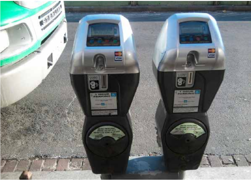
Single-head smart parking meters that accept both credit cards and coins enhance convenience for those that do not carry exact change.
