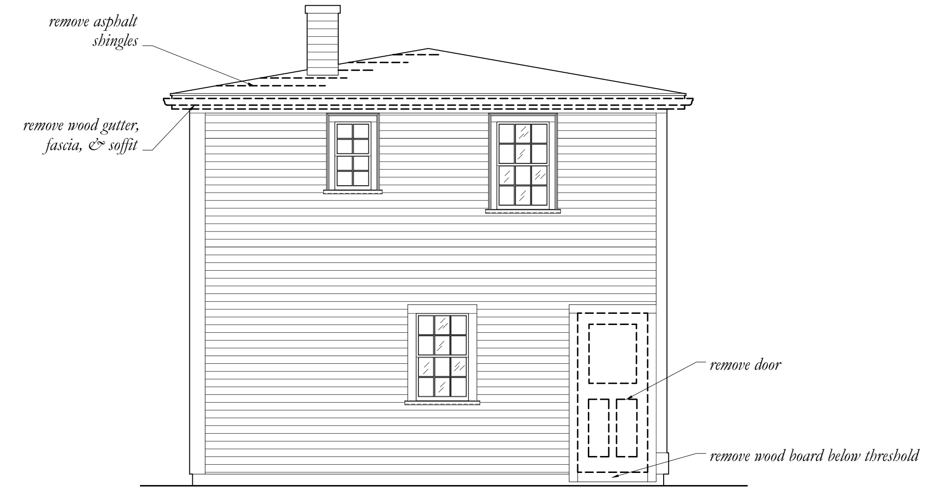
2 DEMOLITION ELEVATION: EAST 1/4" = 1'-0"
