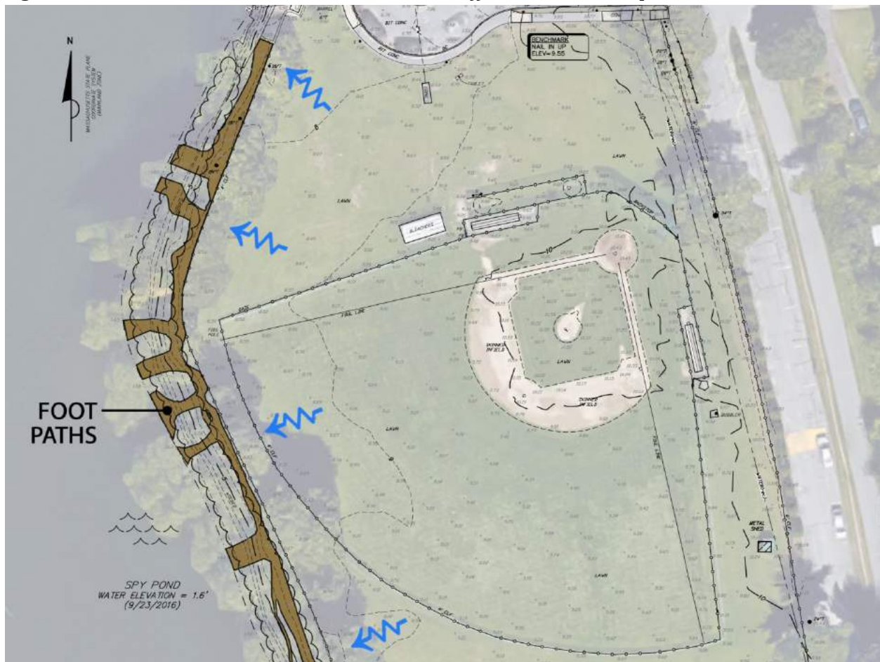
Figure 3– Area1: Scannell Field, Uncontrolled Runoff & Erosion on Slope
