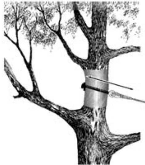
Fig. 33.5.3 Correct cable and hardware alignment
