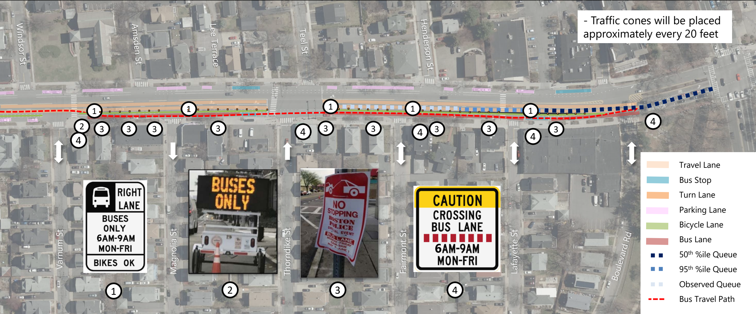
Option 2 – Provide Curbside Bus Lane from Varnum to Alewife Brook Parkway Massachusetts Avenue from Lake Street to Alewife Brook Parkway | Arlington BRT Pilot Project
