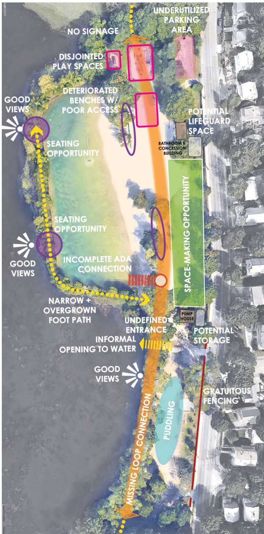
Analysis diagram of the beach and parking area, showing trail conditions, incomplete or non-compliant walking path connections, seating and viewing opportunities, deteriorated perimeter fencing and disjointed programmatic elements
