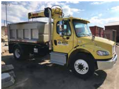
New catch basin cleaner.
