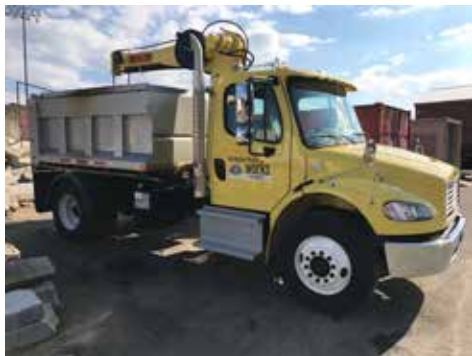
New catch basin cleaner.
