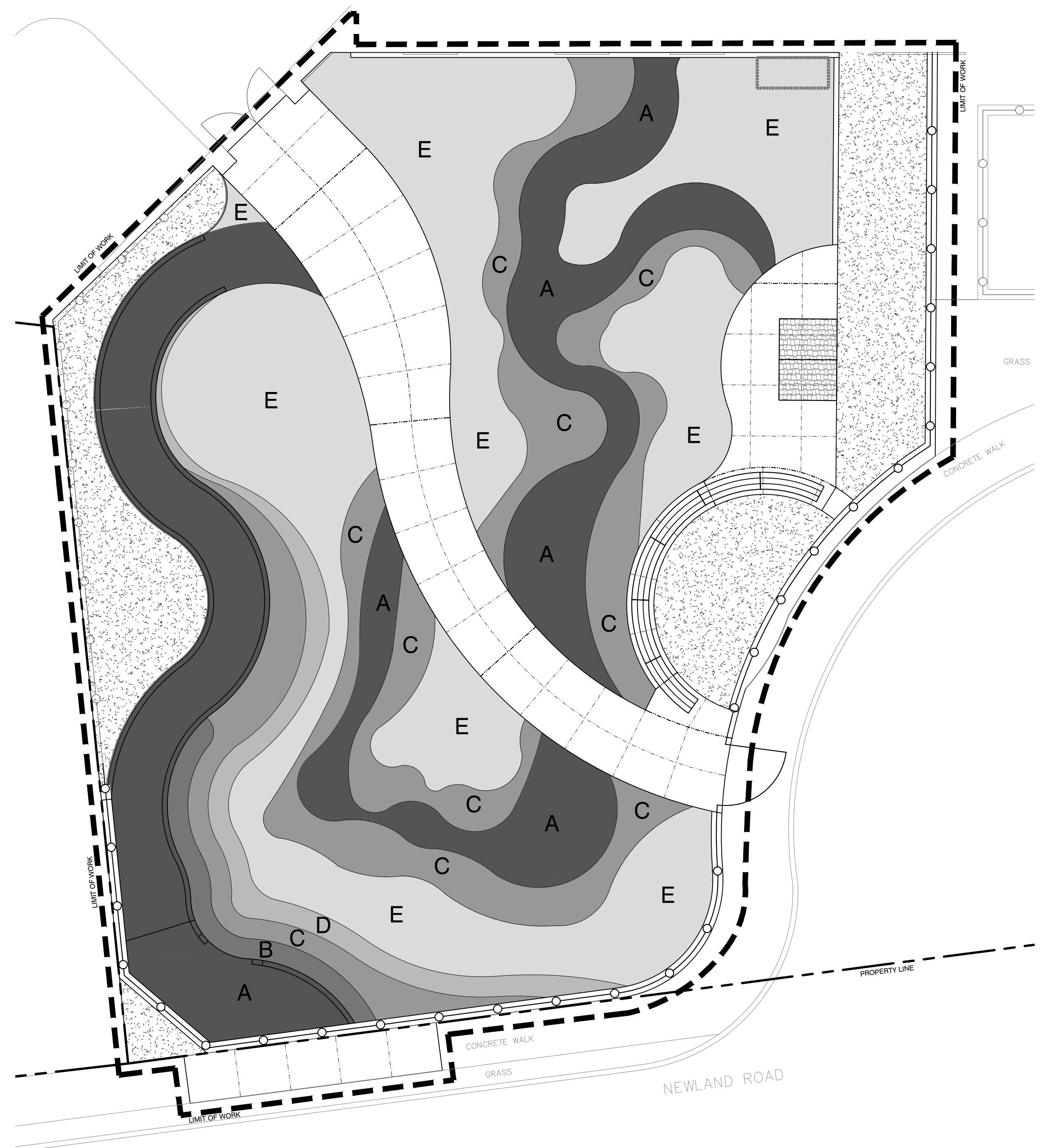
1 POURED-IN-PLACE RUBBER SAFETY SURFACING COLOR LAYOUT SCALE: 1-1/2"=1'-0"
