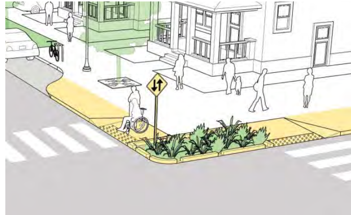
Figure 15. Curb extensions could help shorten crossing distances and slow traffic. Source: NACTO Urban Street Design Guide.
