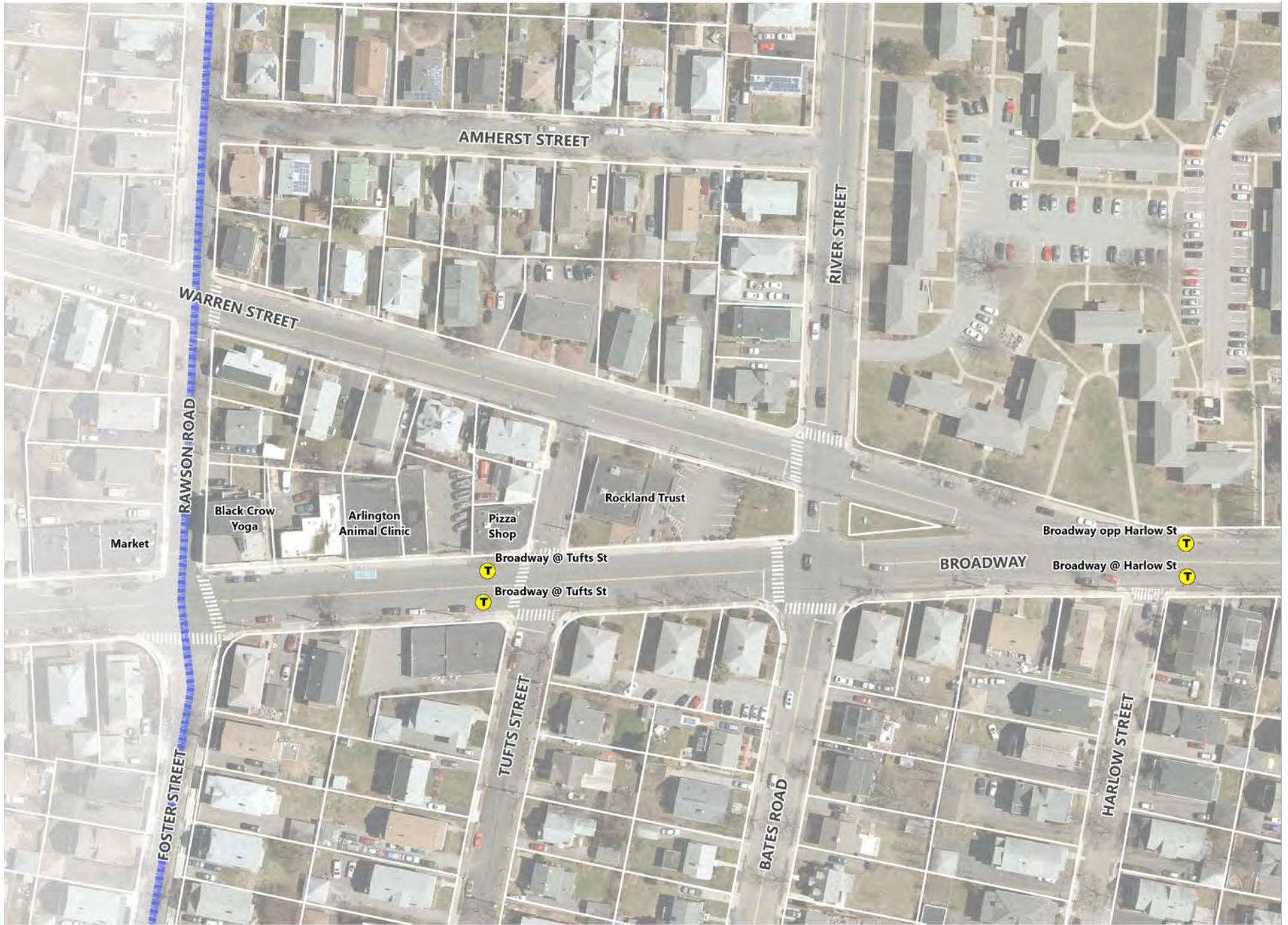
Figure 24. We recommend improving safety at the Broadway/Warren St. intersection through crosswalk safety improvements, signal and/or crosswalk retiming, and painted bike lanes in both directions.
