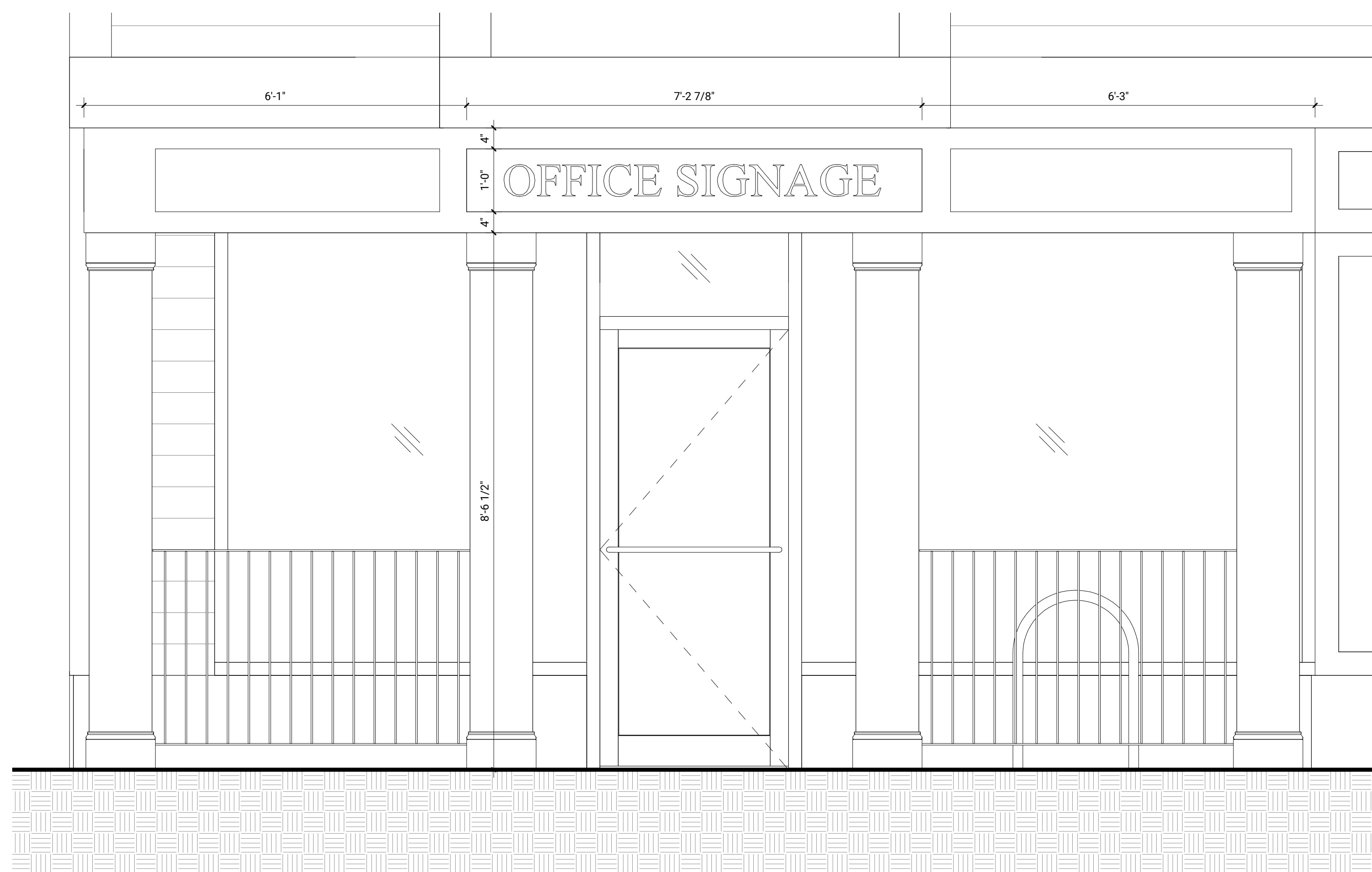
2 ENLARGED ELEVATION - BUILDING SIGNAGE SCALE: 3/4" = 1'-0"
