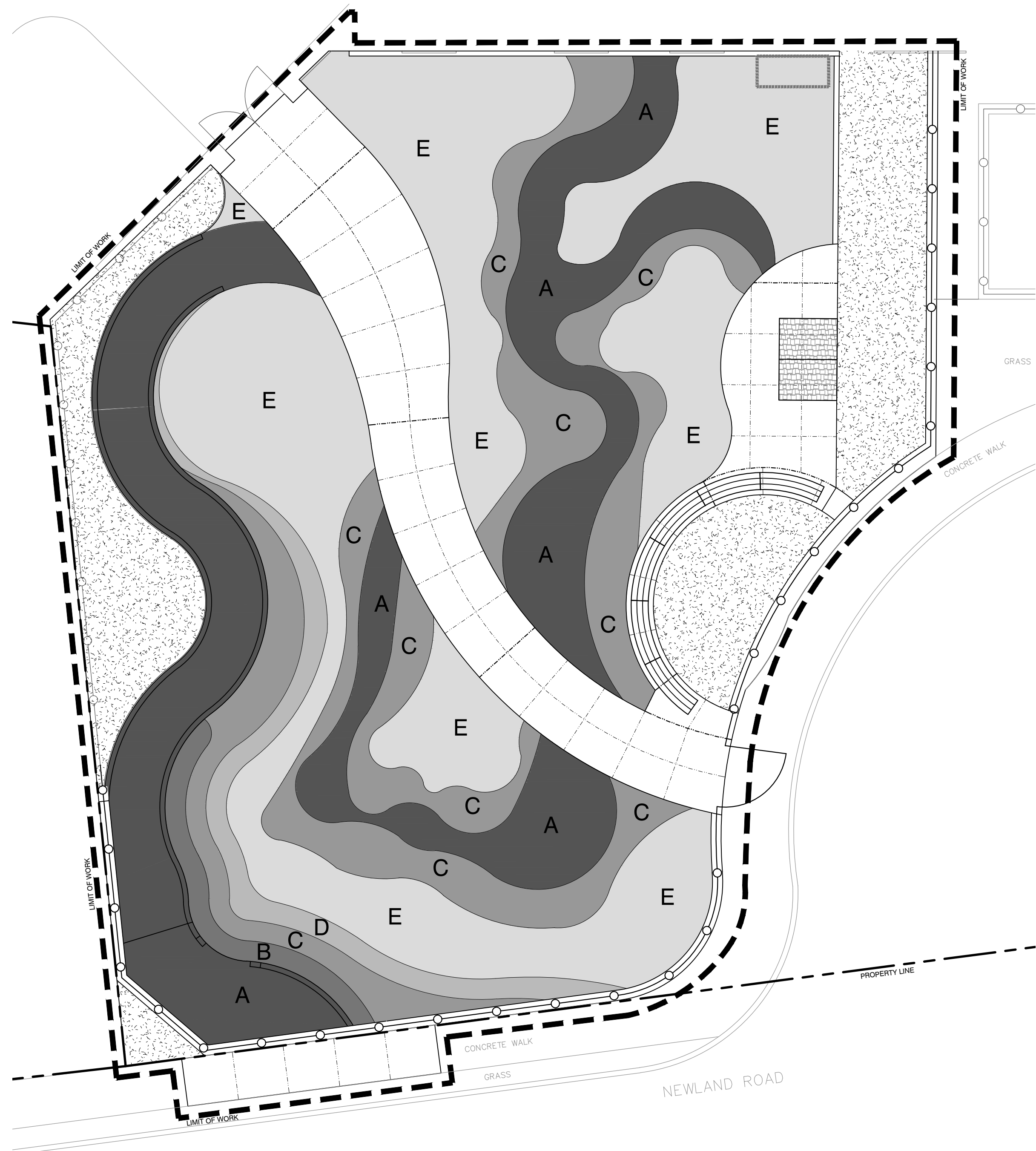
1 POURED-IN-PLACE RUBBER SAFETY SURFACING COLOR LAYOUT SCALE: 1-1/2"=1'-0"
