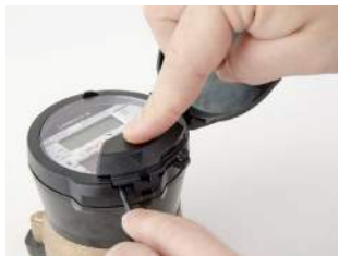
Figure 6 Placing Cover on Register
