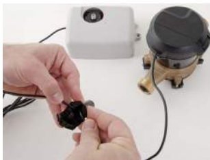
Figure 15 Gray Wires in Slot
