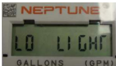
Figure 20 LCD Displaying LO Light
