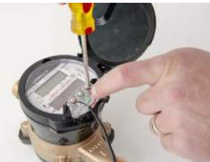
Figure 3 Wiring with Proper Color Wire
