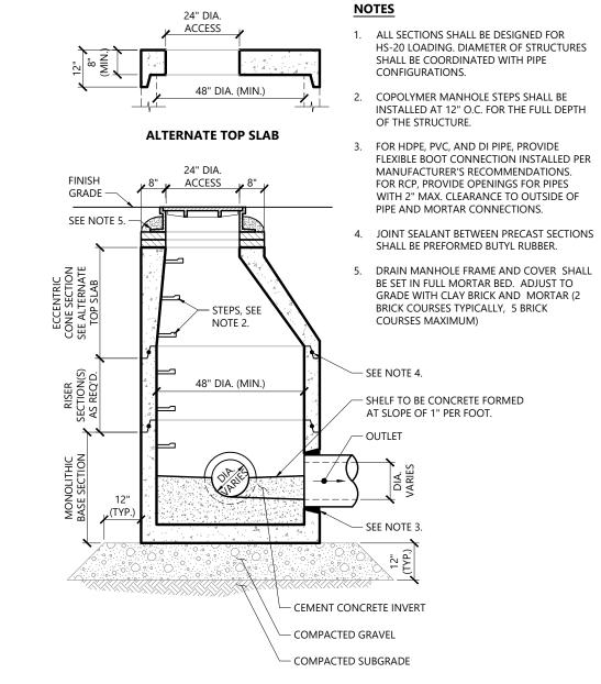
**Drain Manhole (DMH)** Source: VHB
