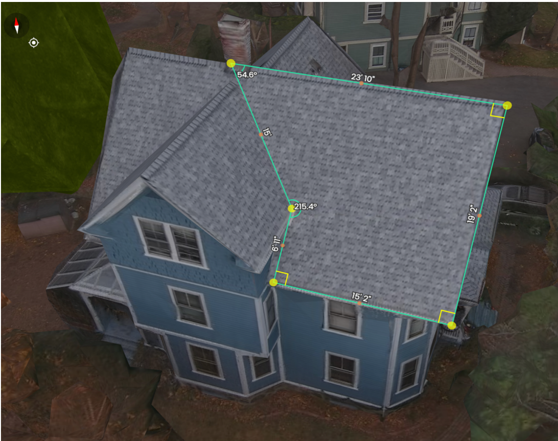
ABOVE: Dimensions of roof plane for proposed solar array. BELOW: "Keep-out" margins for firefighter safety access (18" on ridge)
