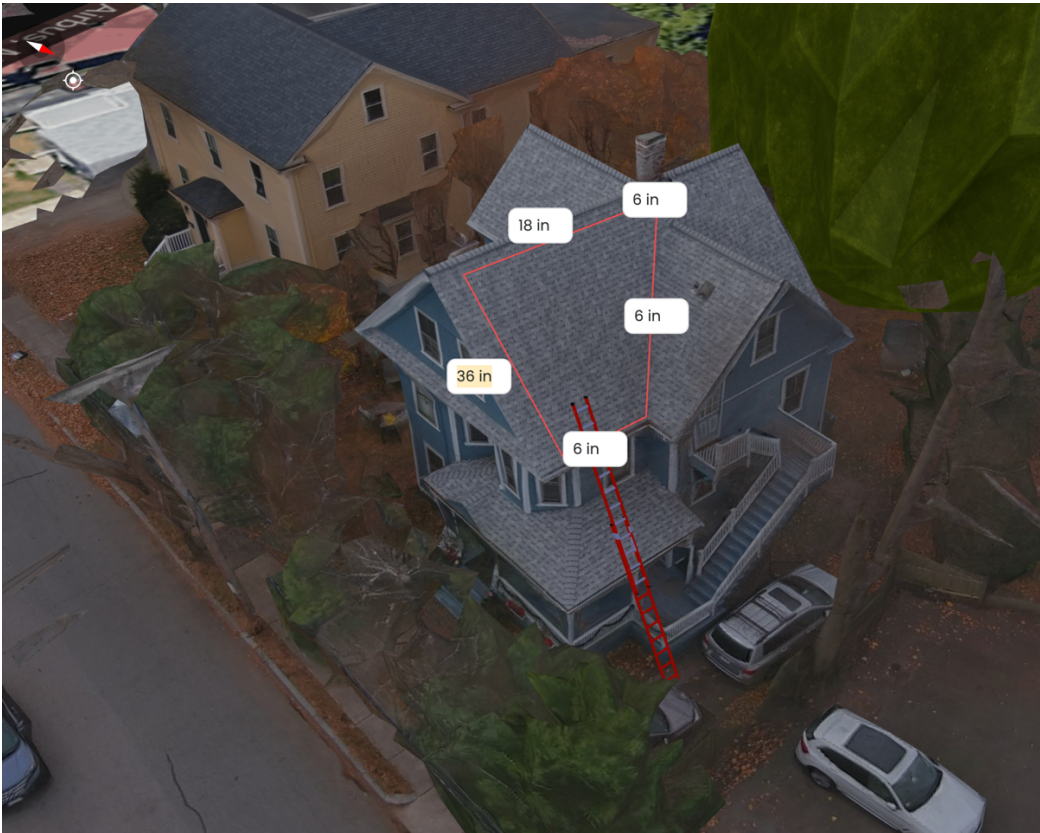
ABOVE: No solar installed on northeast plane - zone shown to demonstrate required safe firefighter pathways (18" at the ridge and at least 36" available inches at the edge to mount the roof).
