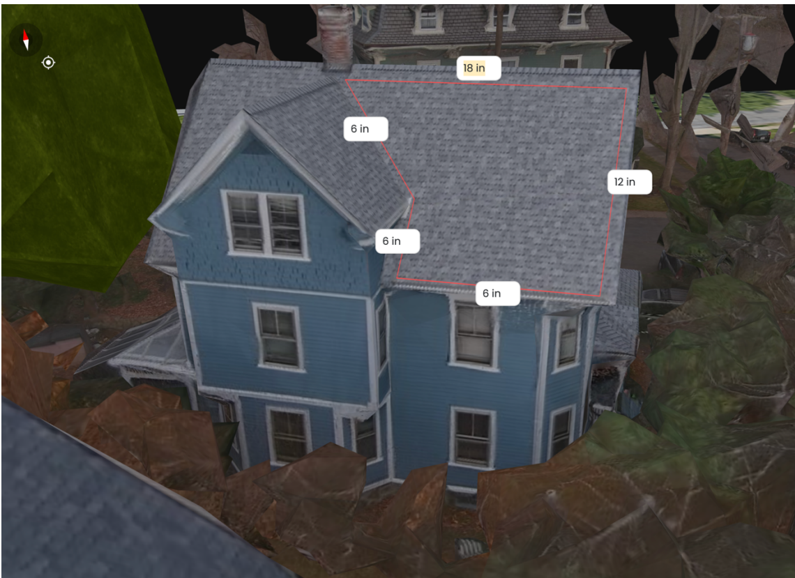
ABOVE: Dimensions of roof plane for proposed solar array. BELOW: "Keep-out" margins for firefighter safety access (18" on ridge)
