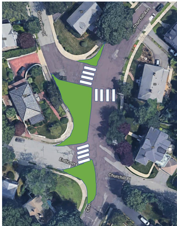
Figure 2: Sketches of alternate intersection design
